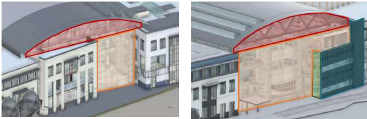
Figure 5. A three-dimensional view of the proposed MPK 12 and 14 lobby atrium. The southeast façade is shown on the left, and the northwest façade is shown on the right. A long-span glazing system will be present in the area shown in red, and insulated glazing is shown in orange and green.
