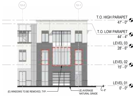
3 PARTIAL MPK 12 SOUTHWEST ELEVATION - EXISTING SCALE: 3/32" = 1'-0"
