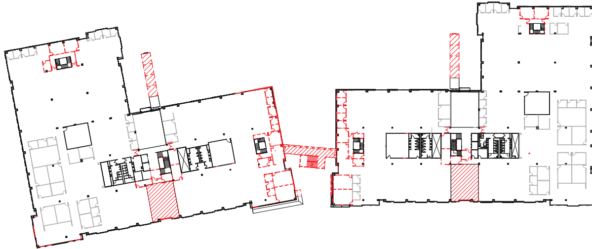
1 MPK 12 & 14 DEMOLITION PLAN - LEVEL 02 SCALE: 1/32" = 1'-0"
