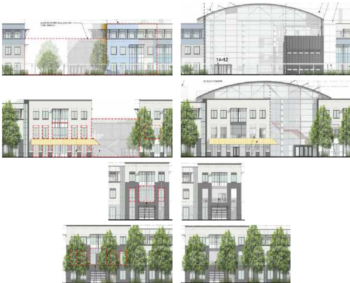
Figure 8. MPK 12 and 14 existing (left) and proposed (right) facades: northwest at lobby atrium (top), southeast at lobby atrium (second from top), southwest at MPK-12 south corner (second from bottom), and southeast at MPK-12 south corner (bottom).
