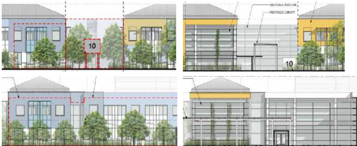
Figure 4. Façade views of MPK 10 showing the existing (left) and proposed (right) facades: southwest (top) showing the southwest side of the new lobby as well as the new connector façade, and east (bottom) showing the east side of the new lobby.
