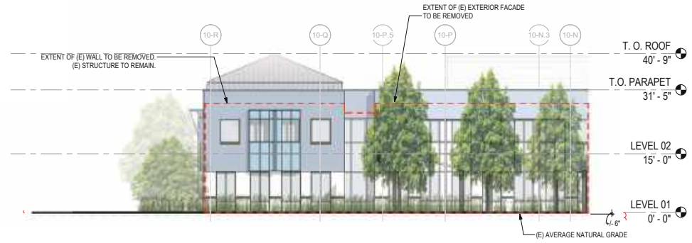
3 MPK 10 PARTIAL EAST ELEVATION - EXISTING SCALE: 3/32" = 1'-0"
