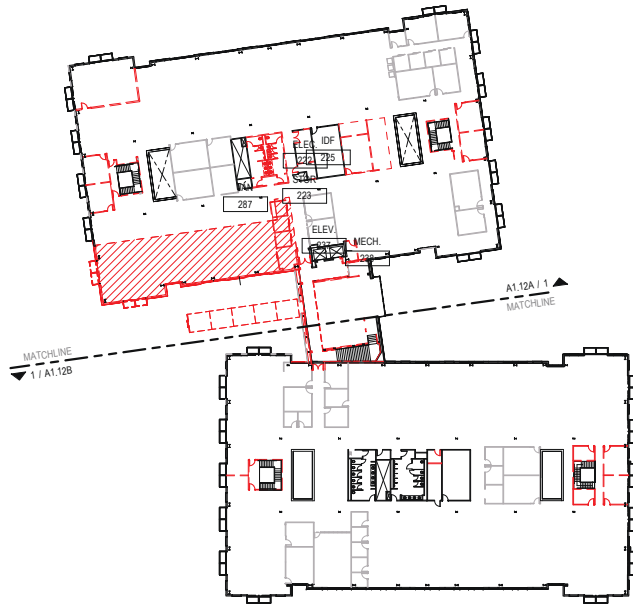
2 MPK 10 DEMOLITION PLAN - LEVEL 02
