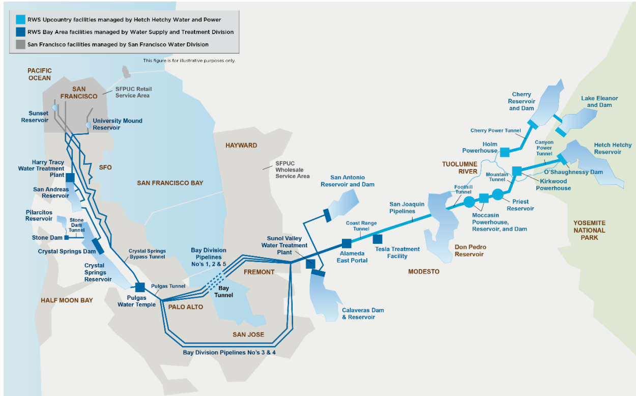
Figure 6-1 Regional Water System and Main Facilities
