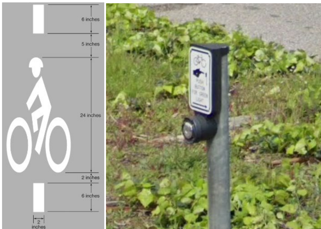
Figure 5-25: Bicycle Detector Pavement Marking and Push Button
