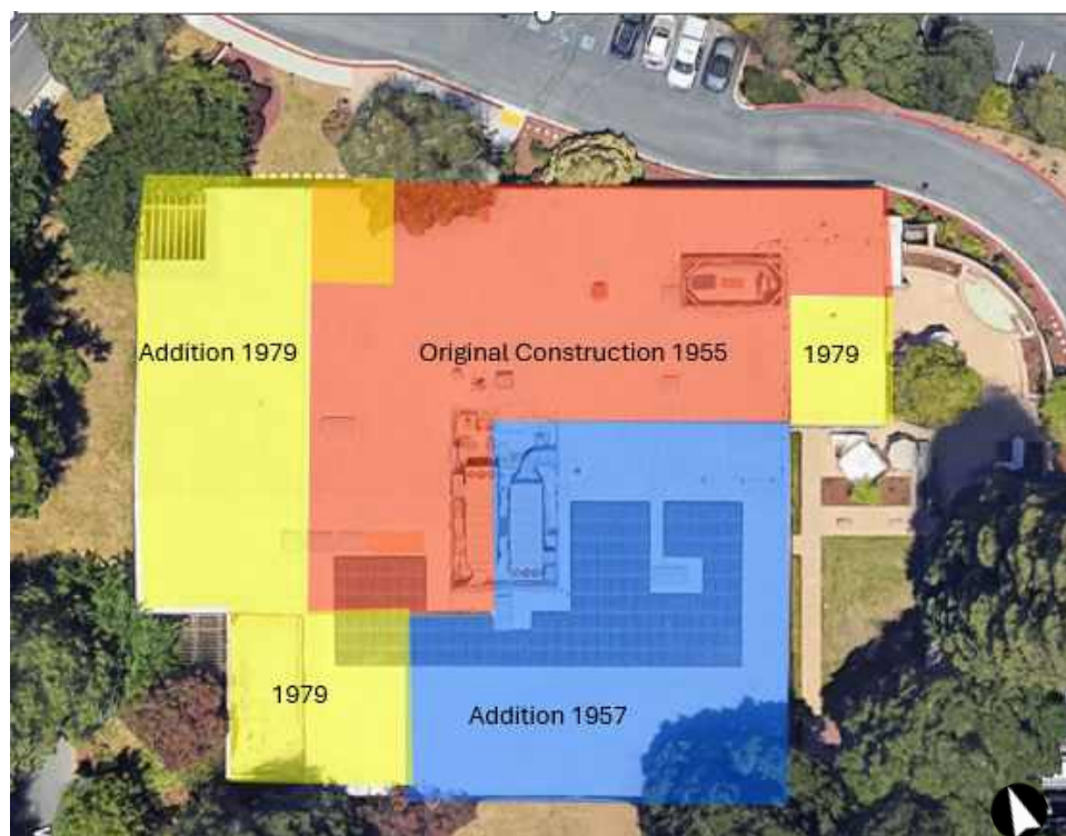
Figure 31: Aerial view showing area of original 1955 construction, shaded red, area of the 1957 addition, shaded blue, and areas of the 1979 additions, shaded yellow. Source: Google Earth 2022. Edited by Page & Turnbull.
