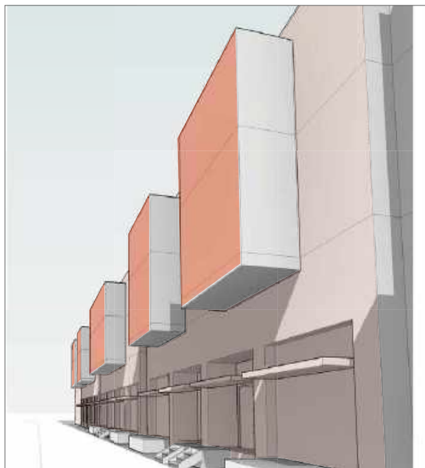
Figure E8. Allowable Building Projection Area
