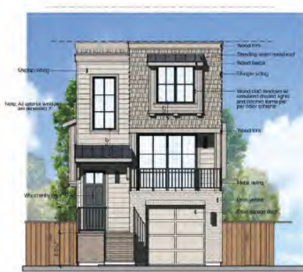
East Elevation (Front)
