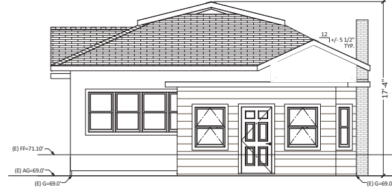
3 EXISTING SOUTH EAST EXTERIOR ELEVATION A0.4 SCALE: 1/4" = 1' - 0"
