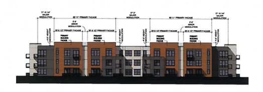
BUILDING #1 & 4 ELEVATION (BUILDING #3 SIM.: SAME MODULATION; DIFFERENT EXTERIOR FINISH)
