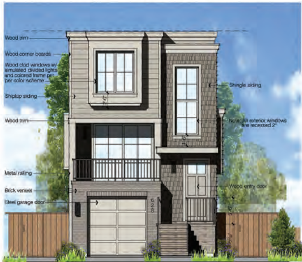
West Elevation (Front)
