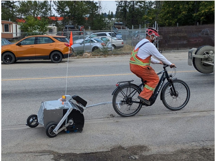
A bike-towed sweeper with a battery-powered brush, run by a municipal crew. Napa County Bicycle Coalition bought one in 2024 for the W. Imola Ave. protected bikeway. Photo: Bike Lane Sweeper Co.
